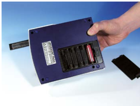
Pic. 11: Battery compartment
